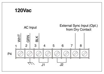
Figure C-1 Wiring the 24A715/M for 120Vac Operation
